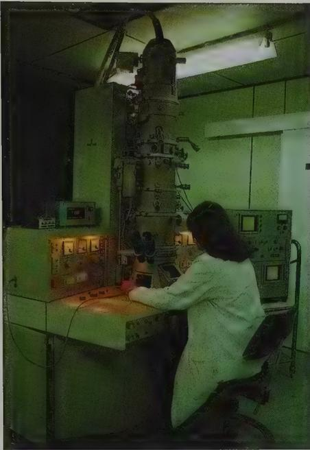
Fig 3.3 A modern transmission electron microscope.
